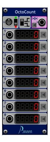
**OctoCount** contains 16 digital counters, separated in two groups. Lower group (channel 1 to 8) is equipped with mono input sockets and with red displays. Upper group (channel 9 to 16) can only used with poly input connector. Their displays are green.
