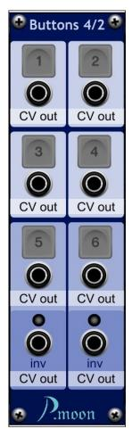
Four push buttons deliver signal while pushed down. Two toggle buttons with both normal and inverted signal out jacks. Output voltage is 5.0 Volts (On) or 0.0 Volts (Off). Labels are editable.
