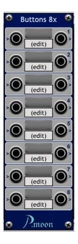
**Buttons 8x** can be used as CV source as well as signal switch. It contains eight push button sections:
