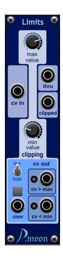
Limits can be either used as signal limiter or only to check signal level.
