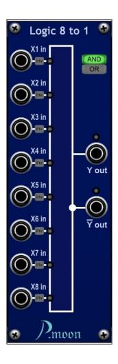
This module works as boolean logic element. It can build an AND or OR result from eight input signals. Every input can be inverted by a toggle button, before signal is displayed and processed.
