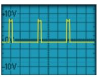
5. Output signal in **min** mode. Signal is always positive.
