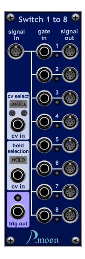
This module switches a poly input signal to one of eight poly output jacks. Selection is done either by *GATE* signals or a *CV* voltage. A *trig out* pulse occurs when a valid selection changes. Hold function can be enabled by a *hold in* signal or a *HOLD* toggle button.
