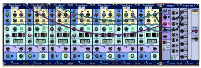
Therefore all *Tone Events's* "arp in" are chained by use of "arp through". "Arp in" of first Tone Event gets "normal clock" in order to get two notes during one step. For a live performance "enable" buttons could be used to activate a double note manually. In this setup a second *Stepper* controls "arp enable" signals. This additional *Stepper* is triggered after last step of main *Stepper* and set to four steps. So four sequences can be a little different from each other.
