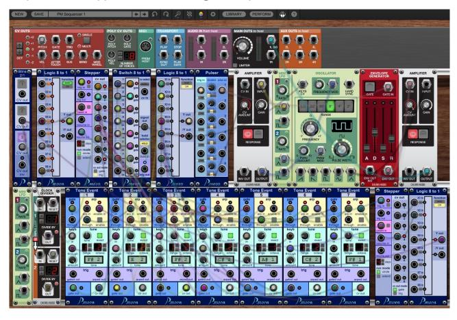
Each *Tone Event* creates both KEYB and GATE signals. Common step sequencers offer just one KEYB and one GATE output. Because this sequencer is modular, there is something to do for getting just this <u>single</u> KEYB and GATE outputs. Therefore additional *P.moon* modules are used as are *Switch 8* to 1 and *Logic 8* to 1.
