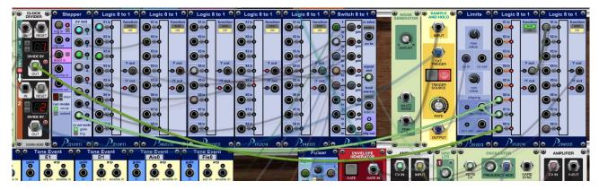
Second GATE part is made to get a ratcheting effect as "illustration". A *Voltage Noise Generator* and a *Voltage Sample and Hold* deliver the random CV. With *P.moon Limits* we can adjust, how often the effect is active. First *Clock Divider*'s output will provide a double note at given steps.
