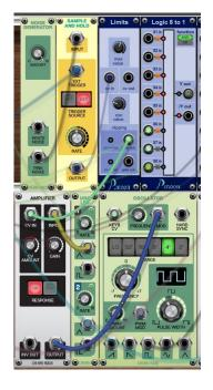
We don't want to get this effect during step 8, when no tone frequency is selected. With AND function of another *Logic 8 to 1* module and inverted step 8 "cv out" this problem is solved.
