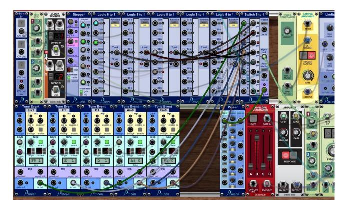
Only *Tone Event*'s "cv outs" are used in this setup. A *P.moon Switch 8 to 1* collects these signals to a single KEYB voltage for the tone oscillator.
