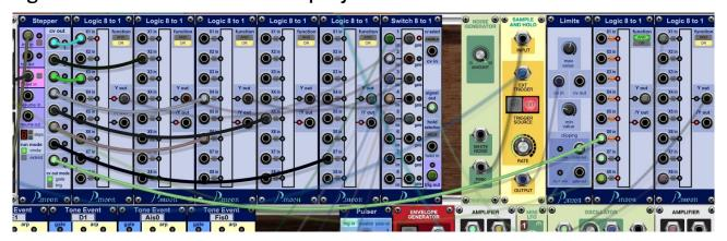
With "gate cv out mode" stepper outputs deliver a gate signal of just one step duration. That is what we need to determine, which tone should be active in which step. P.moon Logic 8 to 1 modules collect all step signals for even one tone frequency.
