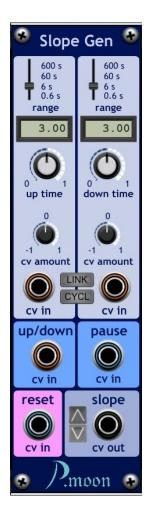
**Slope Gen** is a slope CV generator. Rising and falling slope may have same or different duration from one millisecond up to ten minutes.
