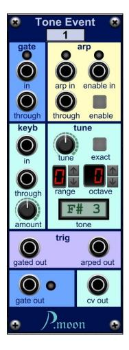
This module can be used both as standalone and as stage of a step sequencer. It provides GATE and CV output signals, that can be used to control any sound source. Together with a **Stepper** module several **Tone Event** modules can form a step sequencer.
